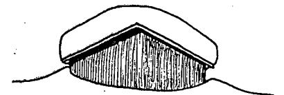
Light, dry snow stays on the roof for insulation effect.
